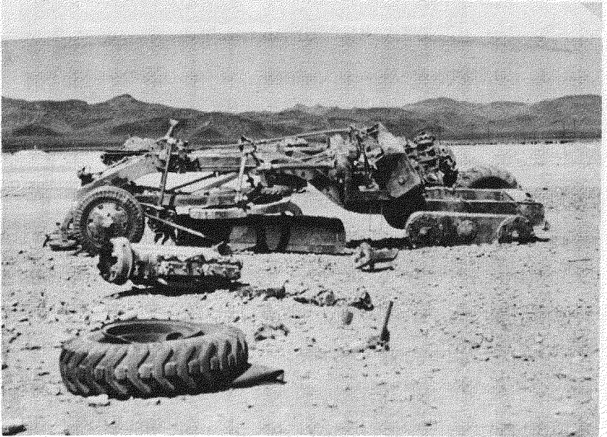
Figure 12.40a. Earth-moving equipment subjected to nuclear blast in open terrain (30 psi overpressure).
